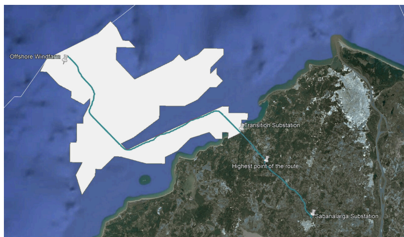
Figure 3. Final transmission route visualized in Google Earth, including both overhead and submarine, and their coordinates.
