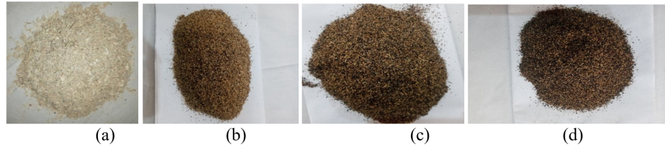
Figure 4. Samples of raw and torrefied blends of corncob and African birch wood residues (a) raw blends of CC and ABW (b) torrefied blend at 240°C (c) torrefied blend at 260°C (d) torrefied blend at 280°C.
