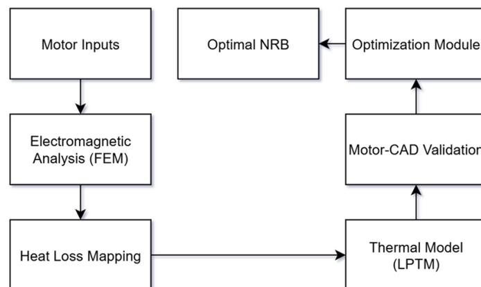
Figure 3. Workflow of the electromagnetic–thermal analysis and optimization process
