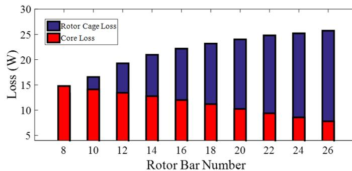
**Figure 28.** Variation of rotor cage and core losses
