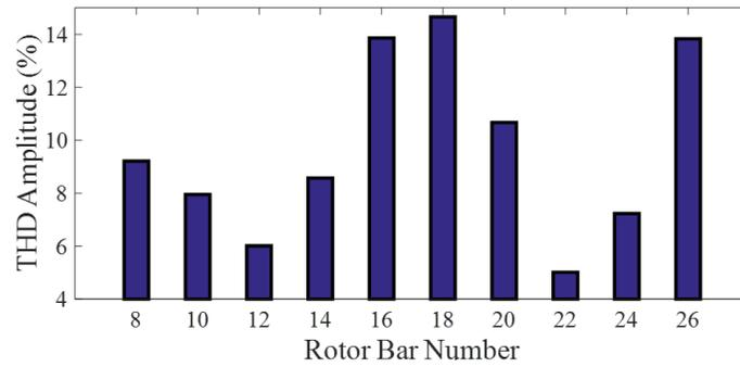
**Figure 5.** Variation of stator current THD
