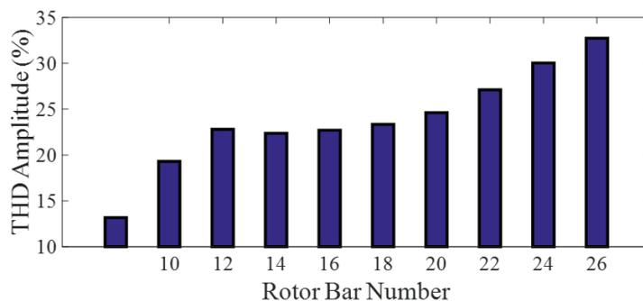
**Figure 21.** Variation of rotor bar current THD
