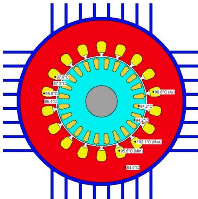
Figure 29. Motor-CAD simulation results in the case of 24 rotor bars
