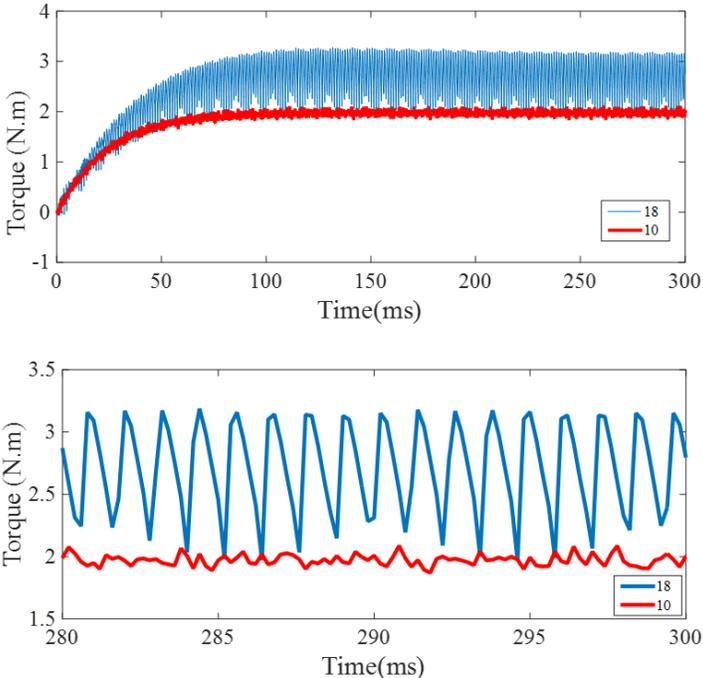
Figure 25. Electromagnetic torque waveforms in the case of 10 and 18-rotor bar
