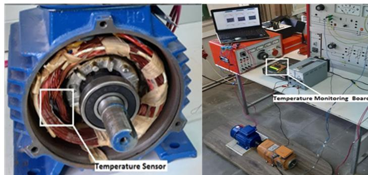
Figure 2. Test bench of IM and temperature metering hardware
