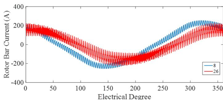
**Figure 22.** Rotor bar current waveforms for 8 and 26 rotor bars
