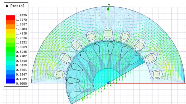
**Figure 1.** IM model in Maxwell software
