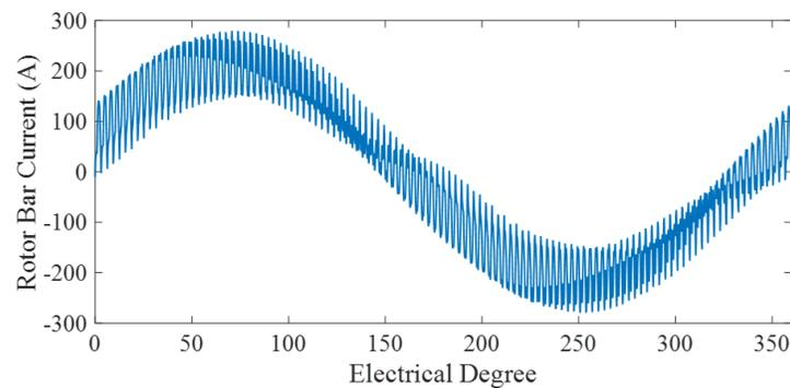
**Figure 9.** Current of rotor bars in the case of 14 rotor bars
