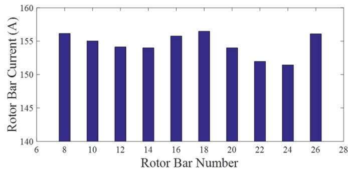
**Figure 7.** Variation of rotor bar current
