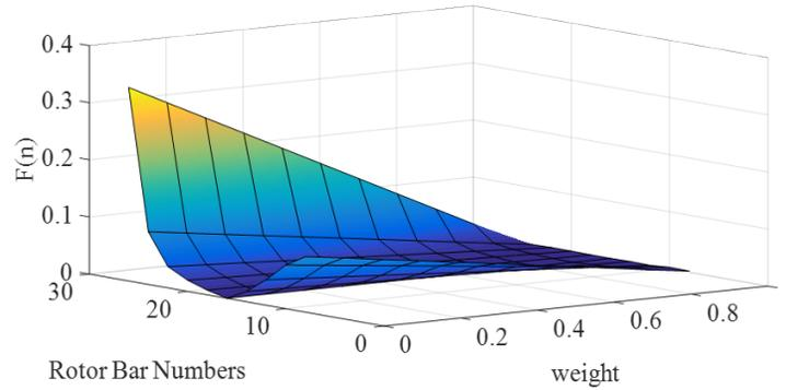
**Figure 18.** Solving optimization function for rotor bar number and desired weight
