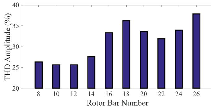
**Figure 8.** Variation of rotor bar current THD
