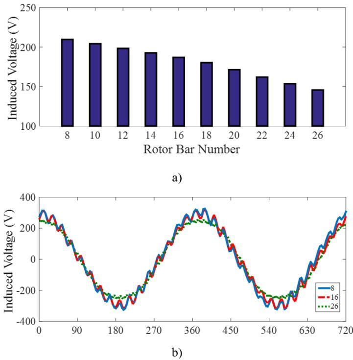
**Figure 19.** The induced voltage in the stator winding (a) RMS value for rotor bar number (b) voltage waveform
