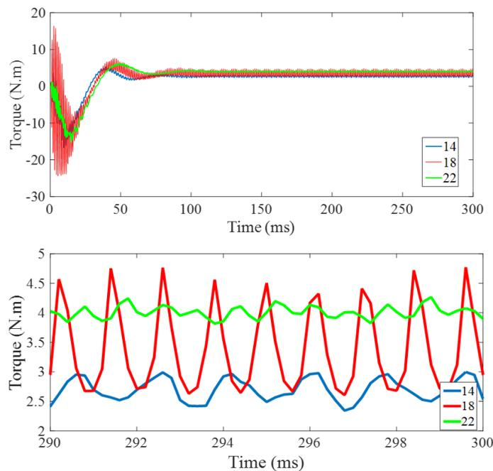
**Figure 12.** Electromagnetic torque waveforms in the case of 14, 18, and 22 rotor bar
