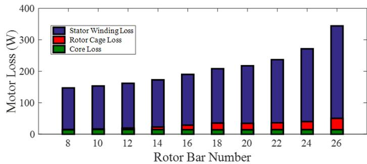
**Figure 15.** Variation of motor losses
