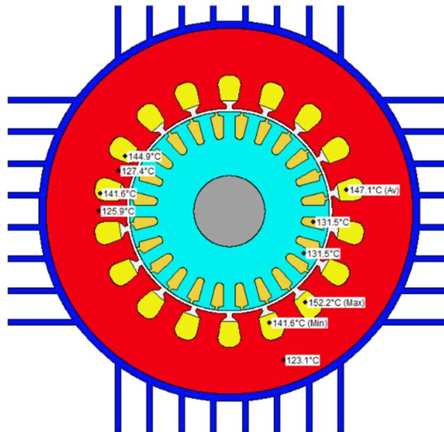
Figure 16. Motor-CAD simulation results in the case of 24 rotor bars
