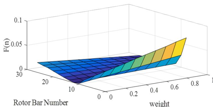
**Figure 31.** Solving Optimization function concerning rotor bar number and desired weight
