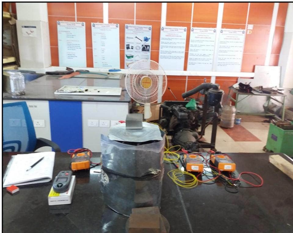
**Figure 25.** Experimental Setup with fins (forced convection).
